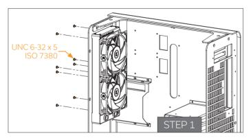
The position of the radiator in the PC case will depend on the size, fan mounting holes, and hardware you have installed. You have to make sure that the radiator and fans fit into the chassis. Usually, the chassis has standard fan mounting holes so you should look for holes with a spacing of 105 mm for standard 120 mm computer cooling fans or 125 mm for 140 mm computer cooling fans.
