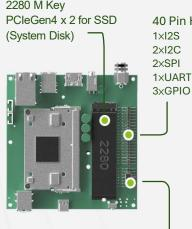
14 Pin Header 1xCAN Bus 1xUART with CTS/RTS 1×UART for Debug 2280 / 3080 M Key PCleGen4 x 4 for 2<sup>nd</sup> SSD / Video Capture CleGen4 x 1 + USB2.0 for BT / Wifi Nano Sim Card Ax 2 Lane
